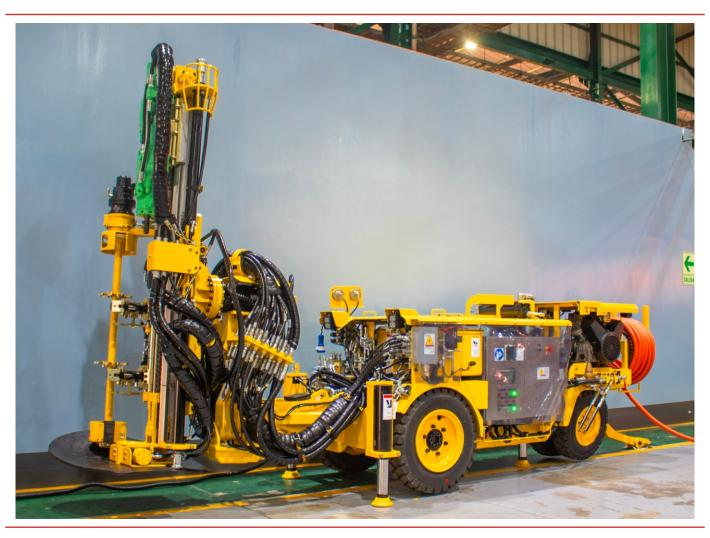
MUKI 22 is an electrohydraulic rig for long hole drilling, just for very small sections; specially designed to be disassembled and entered to drilling work sections throught shafts avoiding the construction of access ramps.
